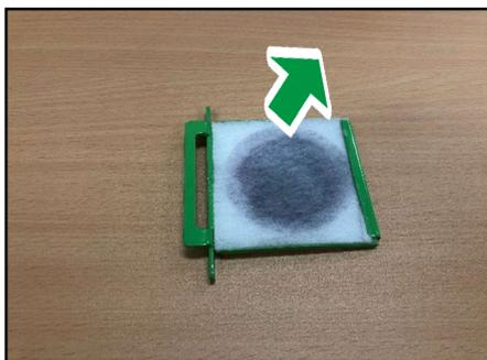
**3.2.4. Set the new mist fan filter into the fixing frame.**
