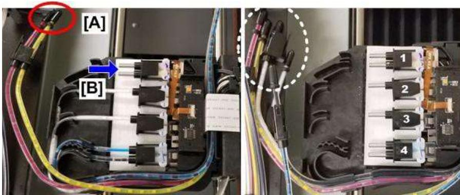
**5.9.23 After you have disconnected all the tubes and plugged the ink ports, you are ready to remove the carriage.**
