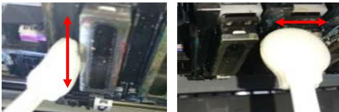
**IMPORTANT!** Do not wipe the protrusion of the Nozzle Cover downward as shown below. The Nozzle Cover may come off causing failure.
