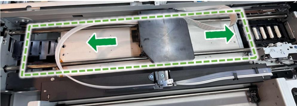
**IMPORTANT!** When moving the carriage, do not enter the area of the maintenance unit.
