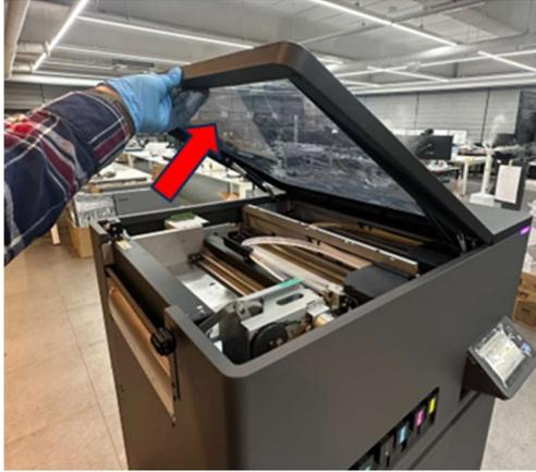
**IMPORTANT!** Do not move the head by hand. It may cause the printer failure.
