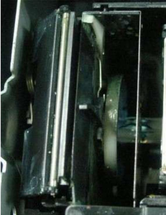
3.6.8.1. Perform cleaning until the surface of the roller, wiper and bottom part of the wiper cleaner are completely visible.
