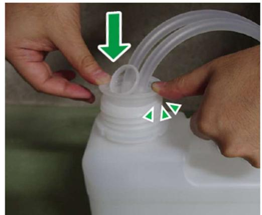
1.4.2. Remove the tape and protector from the waste ink bottle connector, and then connect the waste ink tube to the waste ink bottle connectors on the right back side of the printer.
