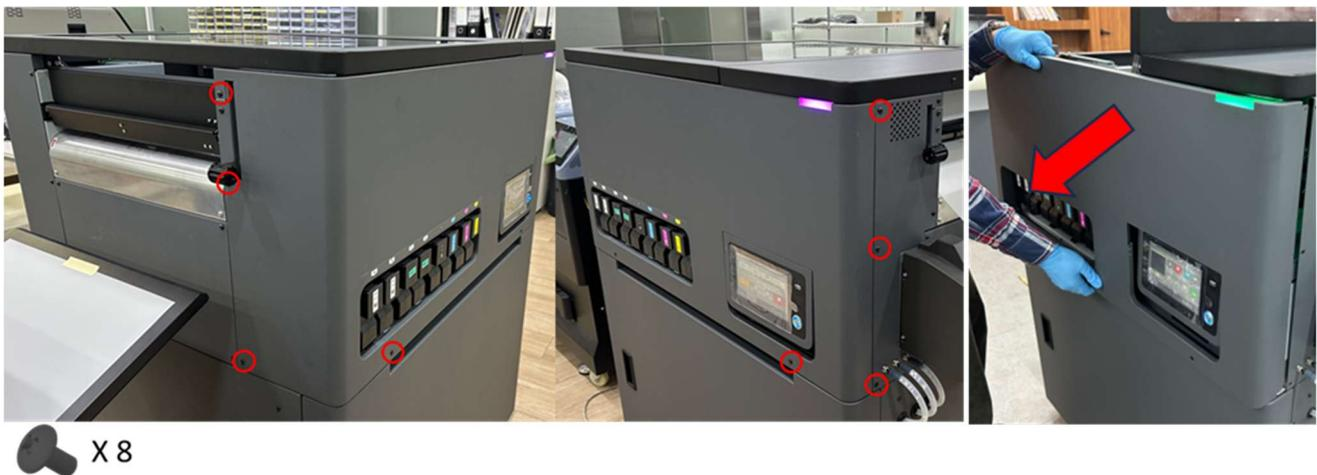
5.4.2. The maintenance unit [A] (and right ink sump below it) are located on the right side of the machine below the carriage unit.
