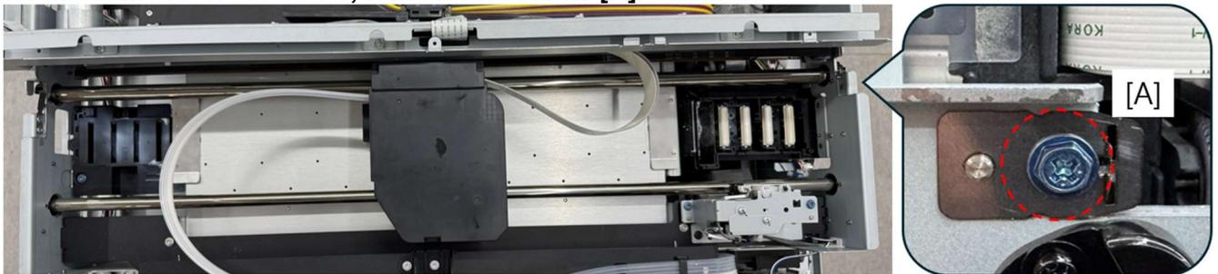
5.9.9. Remove the PLATE holding the ENCODER.
