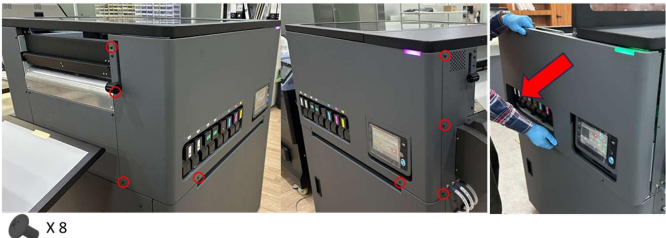
5.6.4. Remove all the printer cartridges.
