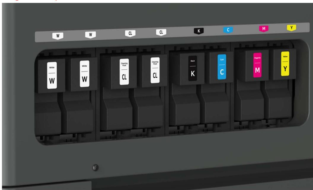
For white ink and cleaning fluid, insert two white ink cartridges and two cleaning fluid cartridges.
