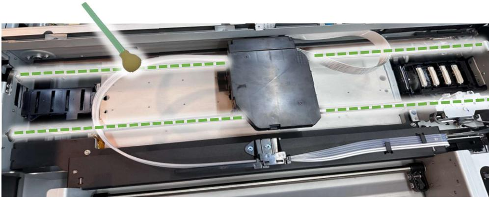
3.5.5. Move the carriage to the left, and then wipe off any old grease and lint on the guide rods where the carriage had stopped.
