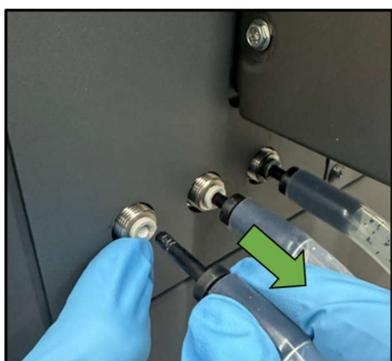
**IMPORTANT!** Do not pull the waste ink tube without pushing the plastic ring.
