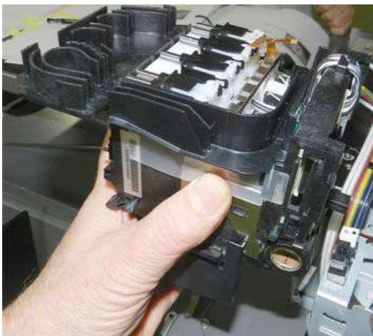
5.9.37. You must connect the FFCs before you can set the carriage in the machine.
