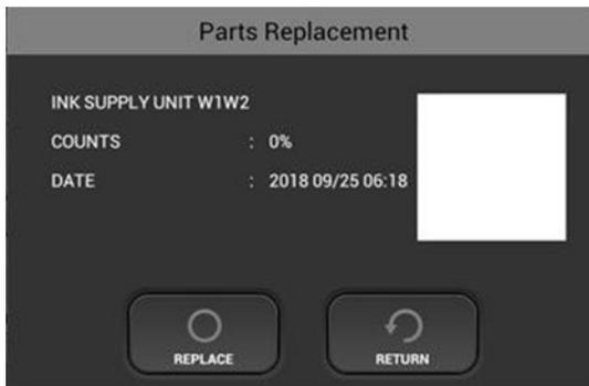
5.6.44. If you replaced more than one unit, repeat Step 5, 6, and 7 for each replaced unit, and then continue to the step below.
