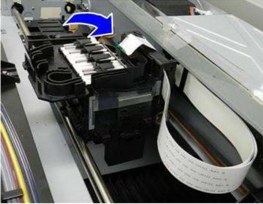
5.9.42. Insert the main guide rod through the bottom of the carriage unit [A], and then into the bushing on the left frame [B].
